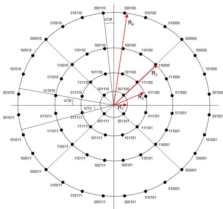
Figure 12: 4+12+20+28APSK Constellation (code rate 132/180)
